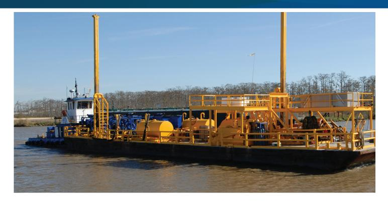
The CM12 is an all-purpose jetting barge that can jet to 20' below the waterline.
